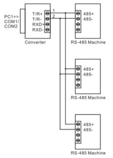
3.Half-duplex communication connections between WI-TOT3201 interfaces
