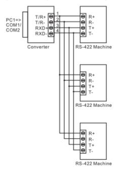
3.Half-duplex communication connections between WI-TOT3201 interfaces
